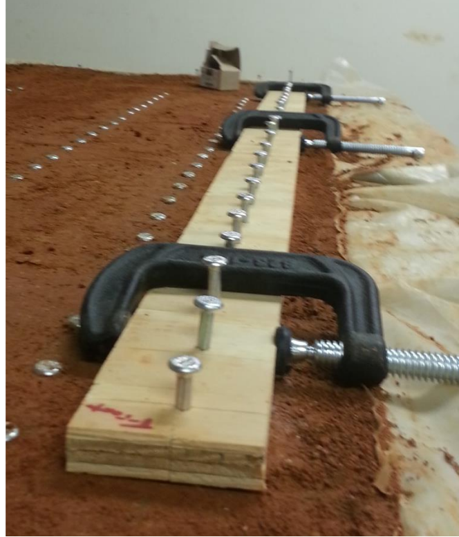
Figure 3-5. Template for placing masonry nails in soil.
