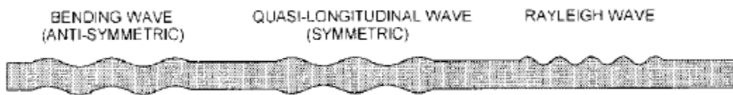
Figure 2-10. Example of Lamb wave particle motion (Ryden et al., 2004).
